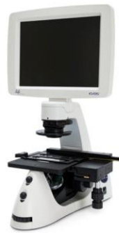
Figure 6. An example of an inverted microscope (EVOS XL core) that can support the correction of displaced tissue.
